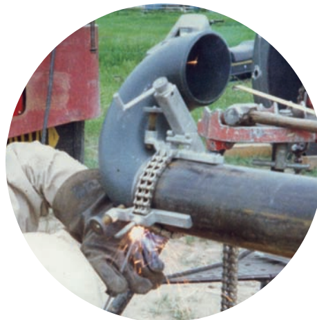
The Mini-Fit Clamp, a miniature version of the Dearman Classic Clamp, is small enough to fit in the welder's tool box.
