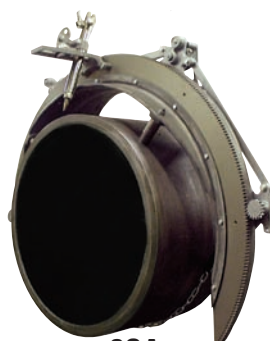
6SA Pipe Size Range 28"-36" / 711mm-914mm
