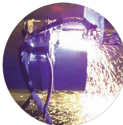
Maxi Chain Machine is rotating a two (2) inch diameter plasma torch around the pipe.
