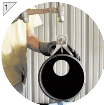
Can be used to measure top dead center.
