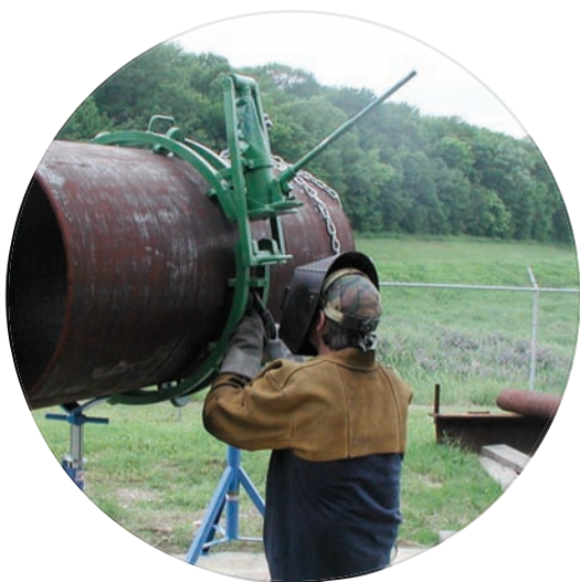
Hydraulic Cage Clamps permit rapid pipe alignment and quick release of the clamp from the pipe after welding.
