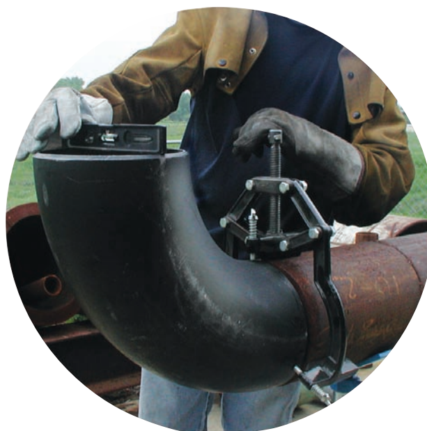
The E-Z Fit Clamp can be used to hold fittings in position for welding.
