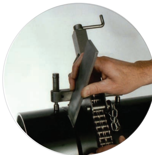
Weld gap can be quickly set using the Spacing Wedge.
